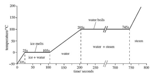
(a) Calculate the energy required to fully melt the ice.
